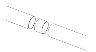
1. The dry installation is joined by putting a 20 gauge split galvanized sheet metal sleeve in between the two butting ducts.
