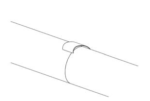
7. After the duct sealant has sufficiently dried, a polyethylene-backed butyl rubber tape is wrapped around the entire joint and screws.
