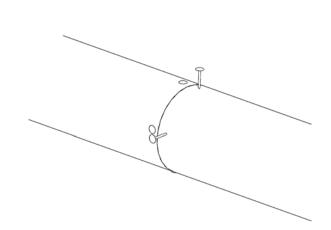
3. The sleeve is then put into the second duct along with duct sealant and screwed into place. The screws are placed 2 inches (2") away from the end of the duct.
