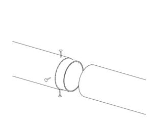
2. The sleeve is put into the first duct along with UL Listed non-hardening waterproof sealant and screwed into place. The screws are placed two inches (2") away from the end of the duct.
