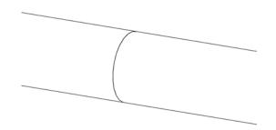
4. Once the ducts and the sleeve are screwed into place, the duct sections should be butted together.
